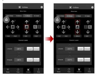
2. Set both extruders to unload temperature (recommend to set the target temperature to 5-10C higher than its normal printing temperature). Unload the filament, and remove the filament and filament guide tubes from the extruder.
