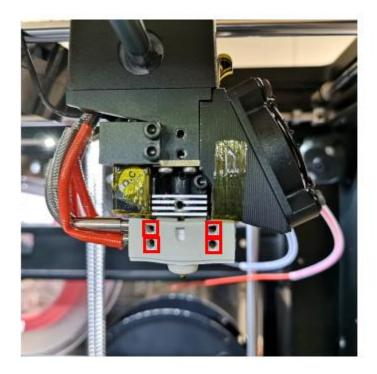
5. Loosen the clamping screw marked in red with 2.5mm hex wrench. Remove the Hot-end from the print head. Take the Heating Rod and Thermocouple out from the Hot-end.
