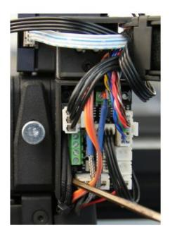
9.Remove the Heating Rod or Thermocoupler from the terminals marked below by loosening the screws with flat head screwdriver on Extruder Board.
